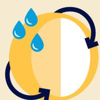
Influenced by soil temperature moisture penetrates the semi permeable E-Max coating and dissolves the nutrient core.
